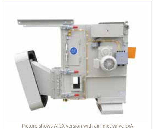
Picture shows ATEX version with air inlet valve ExA
