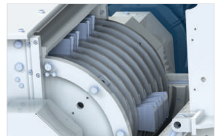
C Robust rotor design with cast material beaters
