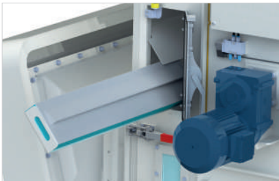
A Upper Magnet can be pulled out for cleaning
