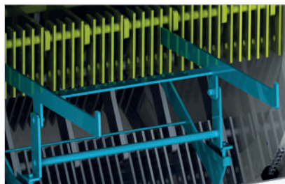
E Beater frame system for quick and easy beater change
