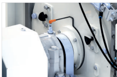
E Bearing temperature monitoring
