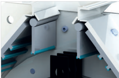
A Inlet flaps and hardened impact plates
