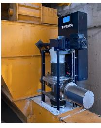
compensation factors on basis of mean values. The OPC will be commissioned on site together with Tietjen service staff that do the training of operators. They learn how to run the OPC in standard applications and how to implement recipe individual adjustments, if necessary.
