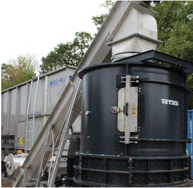
Setup of Biomass Shredder BMS and dosing system from Konrad Pumpe during intensive test period
