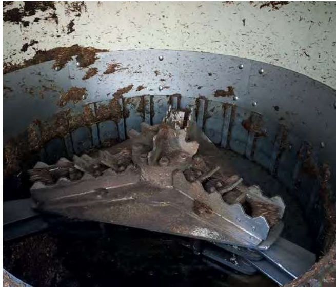
Biomass Shredder BMS: ripping combs for distribution of the material, impact parts and beaters made of wear-resistant materials such as Hardox and carbide
