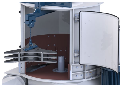
B Crane traverse
