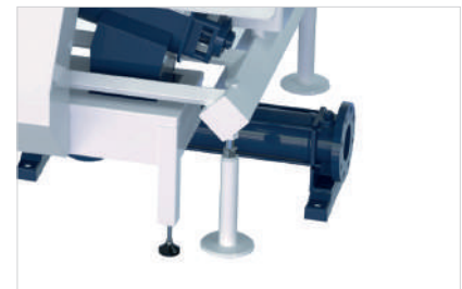
D Pump for transporting the treated organic to the digester
